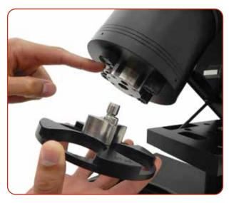
Simple push-button allows easy attachment and removal of sample holders.
