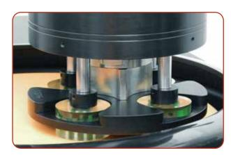
PH-4i<sup>™</sup> individual force configuration: four (4) individual pistons apply force to each mount (1.5" mounts shown).
