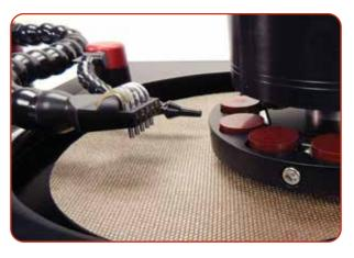
Convenient pivoting arm with nozzle design featuring stainless tips that are easily removed for cleaning.
